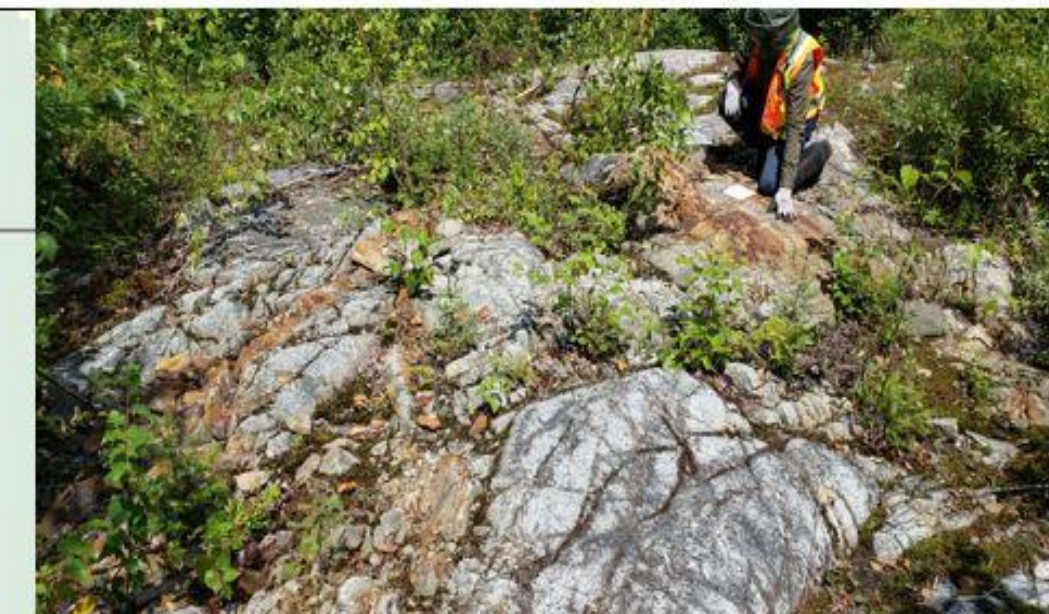
4. 6.0 m wide outcrop at ZamZam zone showing stacked, anastomosing quartz-sulphide veins enveloped by stockworked (breccia) mineralization.. Historical channel samples across the zones 3.41gpt Au / 4.0m and 1.96 gpt Au / 3.70m.
